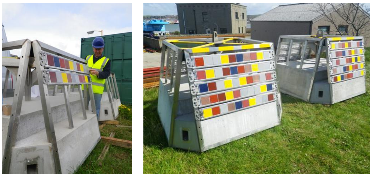
Figure 1: Assembly of the pods and panel units in Orkney.
