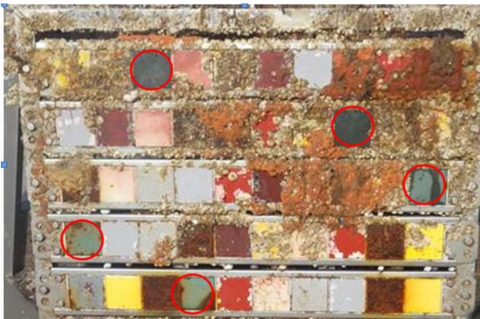
Figure 3: Image of whole pod following recovery in 2017 after 60 months in-situ .
